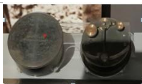
Photo by Fiona Alexander. This instrument was made by von Zatorski from hinges, a mirror, a penny, a safety razor and a brass fuel tank from the primus stove. The cover is on the left.
